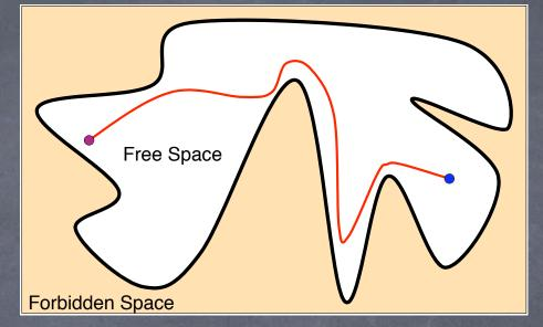
Configuration space (C-Space) -- The space of all the configurations of the robot.
